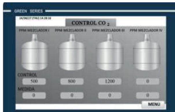
Figure 2. HMI screen showing CO 2 levels and control options for each mixer.
