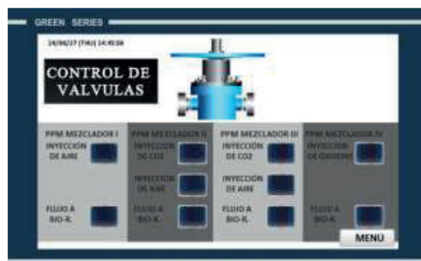
Figure 3. Valve status display indicating active/inactive solenoid valves.
